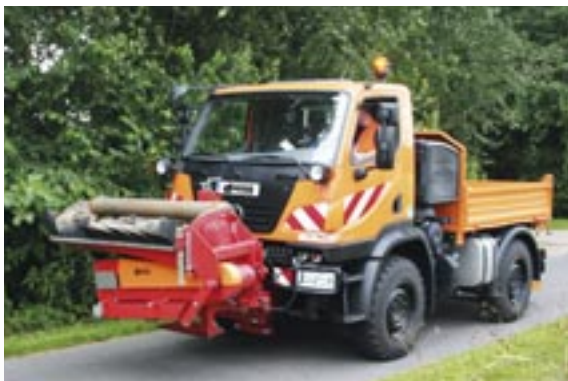
SMT in Transportstellung am Unimog
